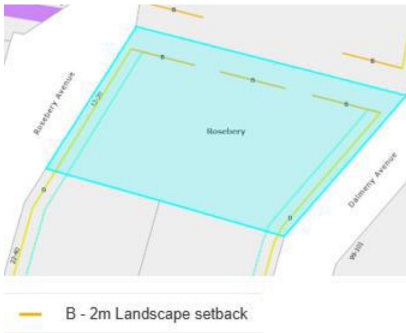
Figure 12: Building setbacks and building setback and alignment map as per SDCP 2012
